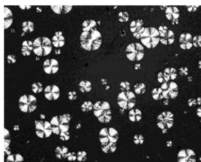
Fig. 5. Photomicrographs of (a) PLLA/PDLA, (b) PLLA/PDLA stereo mixtures added with Talc (1.0 phr) and (c) NA (1.0 phr) in the crystallization processes.
